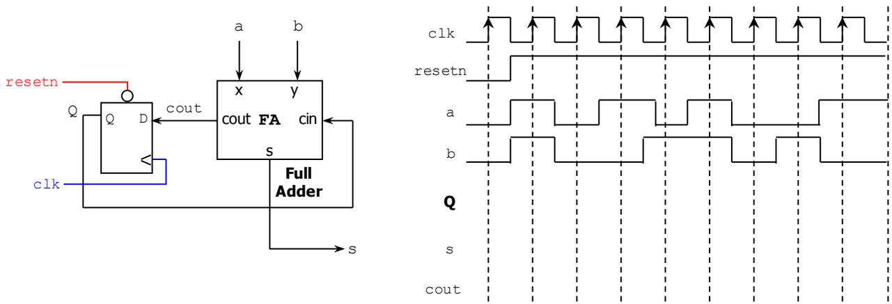
Complete the timing diagram of the circuit shown below. Get the excitation equation for Q. (7 pts)
